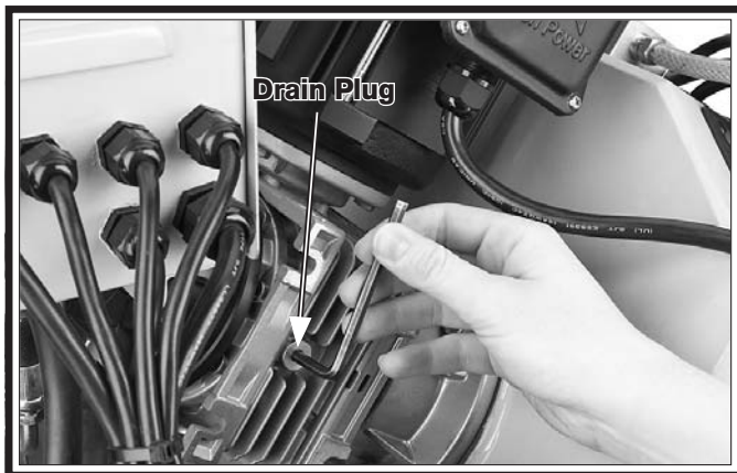
Figure 40. Gear box lubrication.
